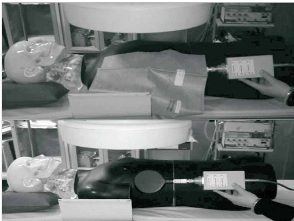
Figure 3. Simulation of radiation exposure with (A) and without (B) the RadPad ® . Image reproduced with permission from Politi et al 34 .
